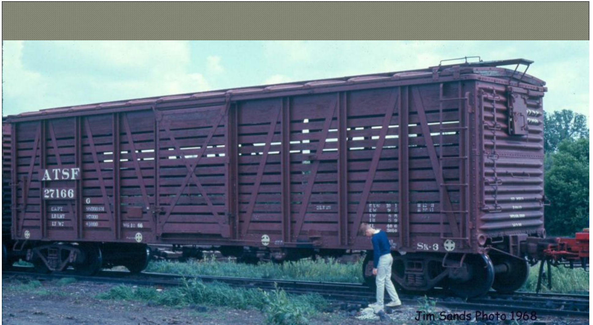
AT&SF 40' wood stockcar with steel ends and roof
