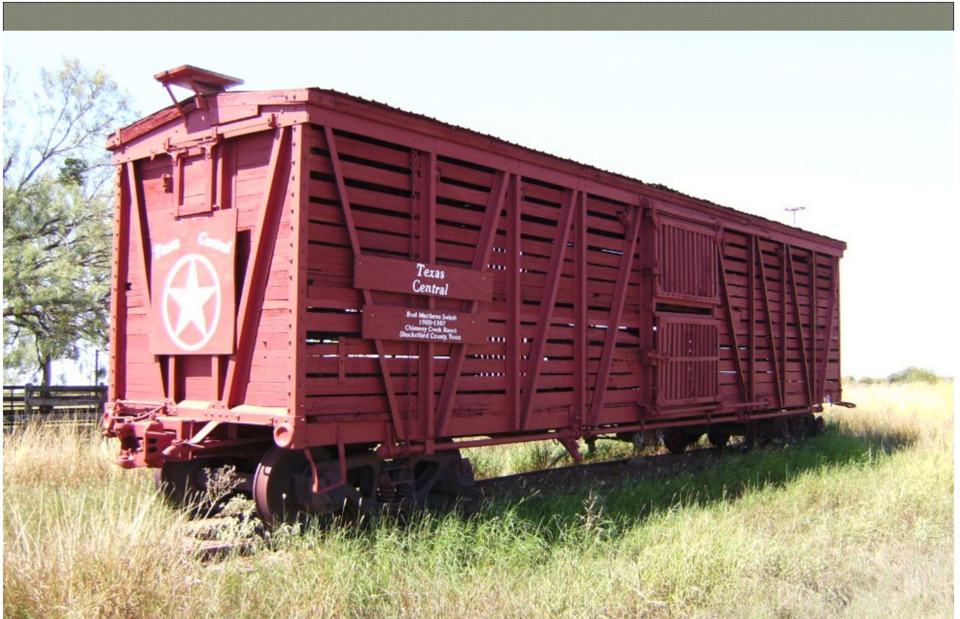
TC convertible stockcar with roller & chain mechanism for raising and lowering the deck
